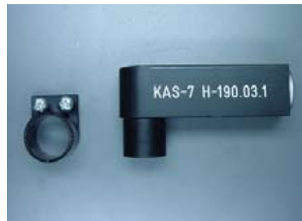
Probe with prism guide KAS-7 H-190.03.1 Angled standard probe for conductivity measurement at 60 kHz
