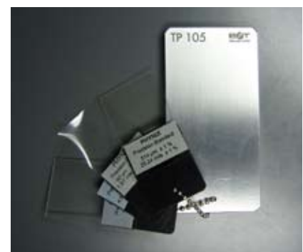
Reference standard TP 105 aluminium Coating thickness standard
