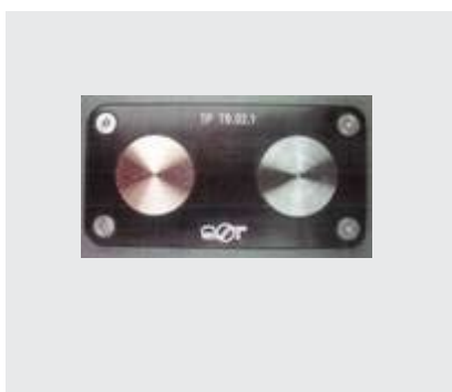
Reference standard TP 79.02.1 Conductivity standard
