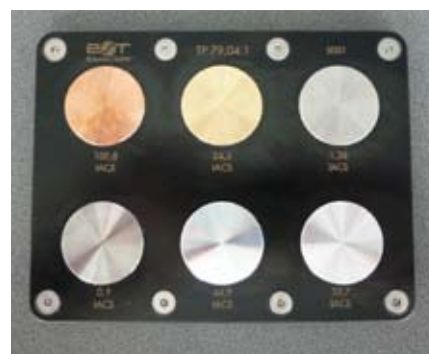
Reference standard TP79.04.1 Conductivity standard
