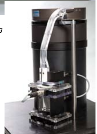
ELOTEST PL500 Q – Sorting Instrument with small sorting system
