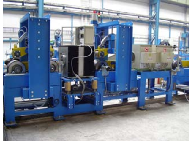
An example of a complete testing line for tubes with the ULAD-coil in M170 magnetization yoke and DC/AC demagnetization.
