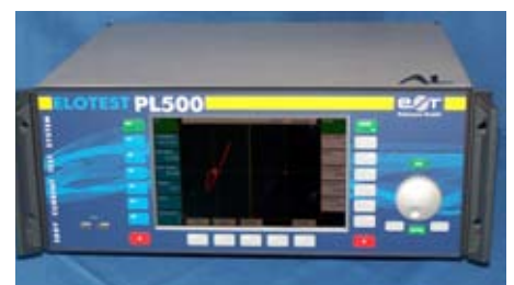
In-Line eddy current test instrument ELOTEST PL500/LP
